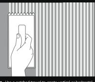
Use a notched trowel to create vertical or horizontal lines in the basecoat prior to the application
