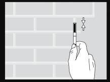
• Cut verticals **TIP** Always cut inwards from corners to avoid broken edges
