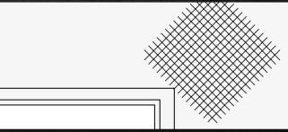
Reinforcing mesh patches should be cut into 200-300mm squares or rectangles and applied to all stress points.
