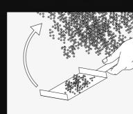
Dash aggregate must be evenly applied to Dash Receiver of correct consistency
