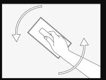
Work the silicone render in small circular motions to remove excess material and create a natural random finish
