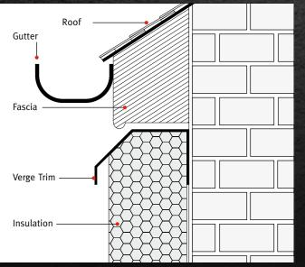
Verge profiles are designed to protect the system on gable ends and roof lines when the system being applied will extend beyond them
