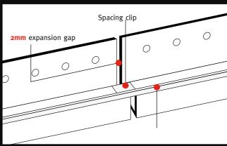
• Clip on plastic nose, placed over joints between each Base Track as a bridge to help reinforce and cover the joint
