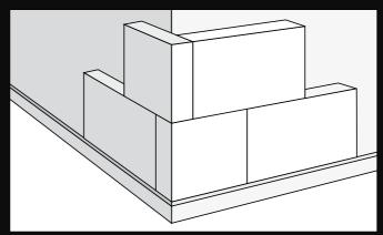
Insulation Panels should always be butted seamlessly together to ensure no gaps exist between them. Take care to stagger joints at the corners of surfaces being covered
