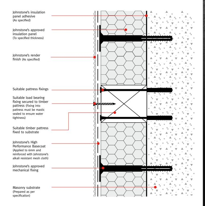
Detail Section: Fixing Brackets (General to heavy load bearing)
