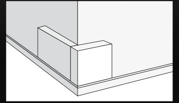
Always fix insulation boards to walls from the base track upwards, starting from a corner
