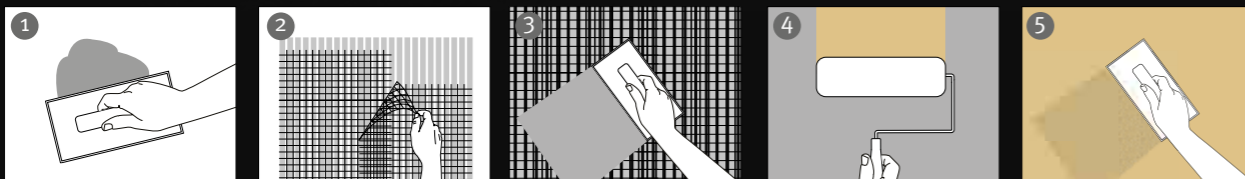
1 Apply Stormshield High Flex Basecoat to suitably prepared substrate 2 Bed reinforcing Stormshield Mesh Cloth into Basecoat 3 Apply second pass of Basecoat to enclose Stormshield Mesh Cloth and to a total thickness of 6mm and work to a plain faced finish 4 Apply 1 coat of Stormshield Silicone Enhanced or Full Silicone Primer to fully cured based coat and allow to dry 5 Apply Stormshield Silicone Enhanced or Full Silicone Render in the aggregate size chosen and finish with a plastic float
