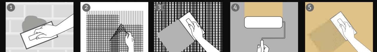
1 Apply Stormshield High performance Basecoat to suitably prepared masonry substrates 2 Bed reinforcing Stormshield Mesh Cloth into Basecoat 3 Apply second pass of Basecoat to enclose Stormshield Mesh Cloth and to a total thickness of 10mm and work to a plain faced finish 4 Apply 1 coat of Stormshield Silicone Enhanced or Full Silicone Primer to fully cured Basecoat and allow to dry 5 Apply Stormshield Silicone Enhanced or Full Silicone Render in the aggregate size chosen and finish with a plastic float
